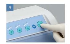
Press the start key. In less than a few moments all handpieces are correctly cleaned and lubricated.
